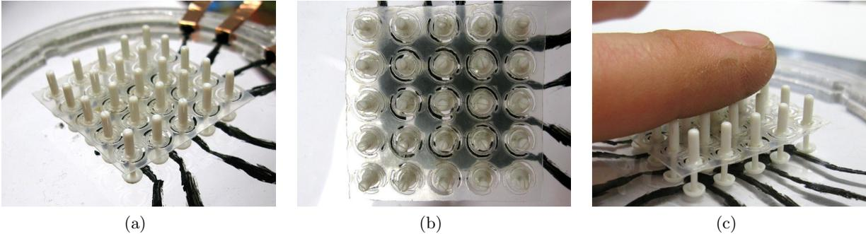
Figure 5: Prototype DEA shear tactile display with  $5 \times 5$  pins in a rectangular grid. The pin spacing is 7 mm.
