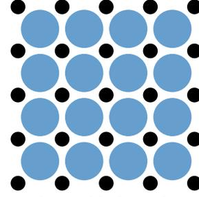
Figure 4: Layout of pins (black) and actuating electrodes (blue/lighter shading) for the prototype.
