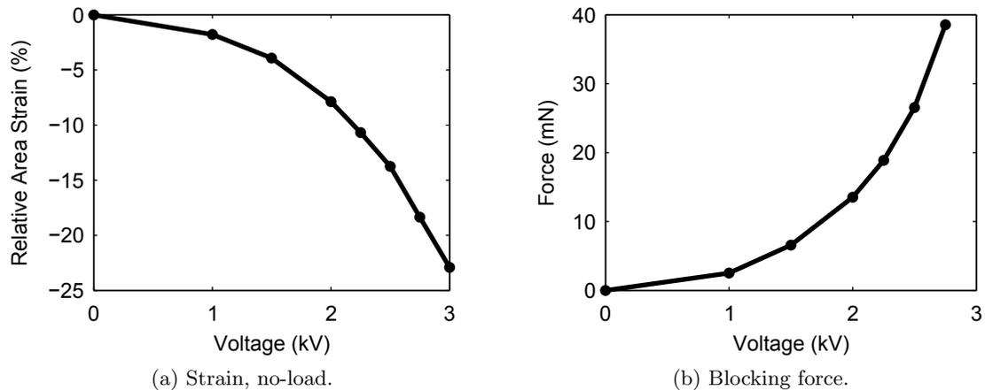
Figure 6: Force and strain against voltage for the characterised prototype.
