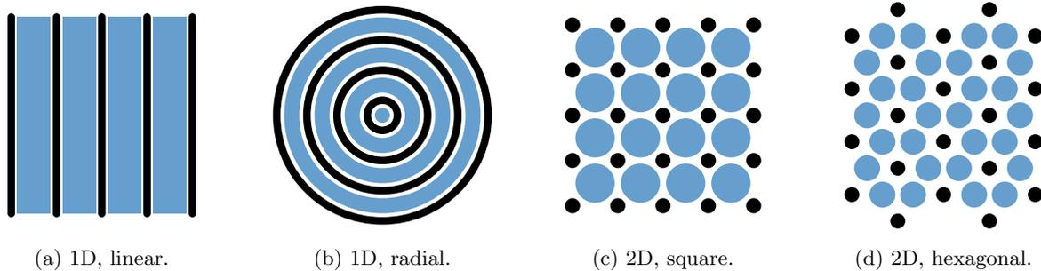
Figure 7: Possible topologies for 1-dimensional and 2-dimensional laterotactile displays. Finger-stimulating elements are shown in black and DEA electrodes are shown in blue/lighter shading.
