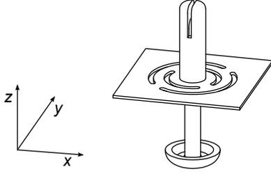
Figure 3: CAD model of a single element of the developed tactile display. The flexural hinge plate gives the pin 2 rotational degrees of freedom.
