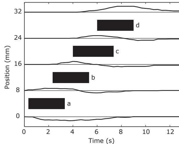
**Figure 6:** Displacement of the tactile bars for a stroke travelling across the device. Black boxes indicate actuation of the respective SMA wires.
