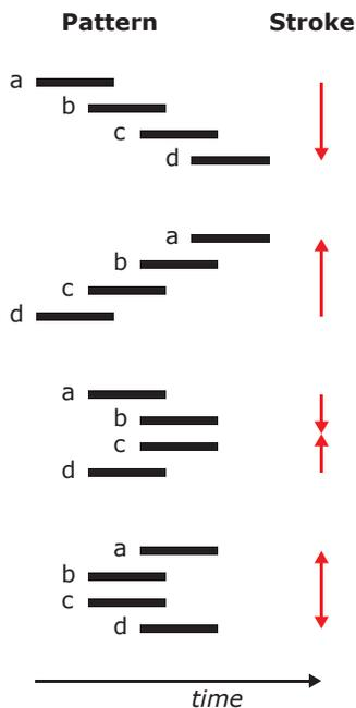
**Figure 5:** Some possible actuation patterns and resulting strokes.
