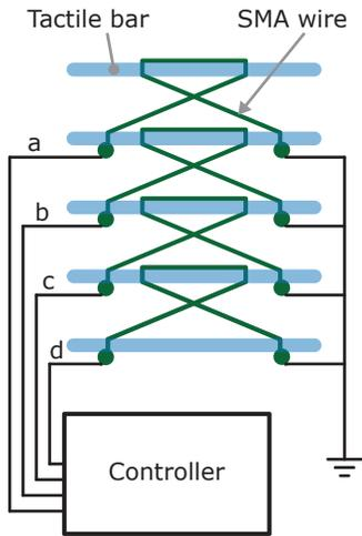
**Figure 2:** Schematic of the configuration of the SMA wires. The crossed pattern amplifies the movement of the tactile bars.
