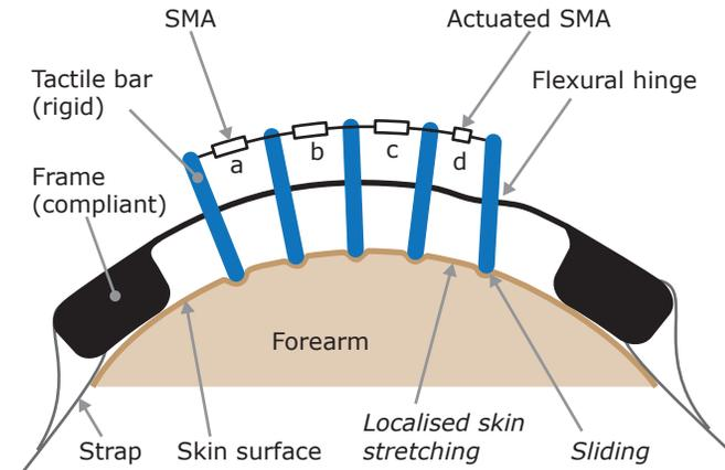
**Figure 1:** Schematic diagram of the Tickler. Actuation of the Shape Memory Alloys (SMAs) cause the tactile bars to move laterally against the skin, which we hypothesise causes *sliding* and *localised skin stretching*.
