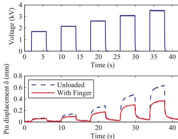
**Figure 10.** Mean displacement of single pin  $\delta$  over time, computed from the area enclosed by the four pins.
