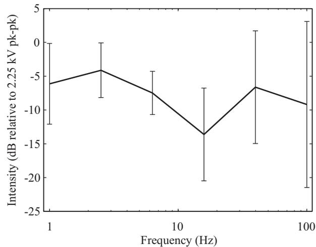
**Figure 12.** Mean absolute sensitivity threshold (dB relative to 2.25 kV pk-pk) from psychophysical study, for frequencies between 1–100 Hz. Error bars show 1 standard deviation.
