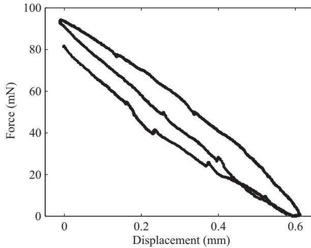
**Figure 6.** Force:displacement relationship of pin 1. The DEA was actuated at 3.5 kV, and pin 3 was mechanically grounded.
