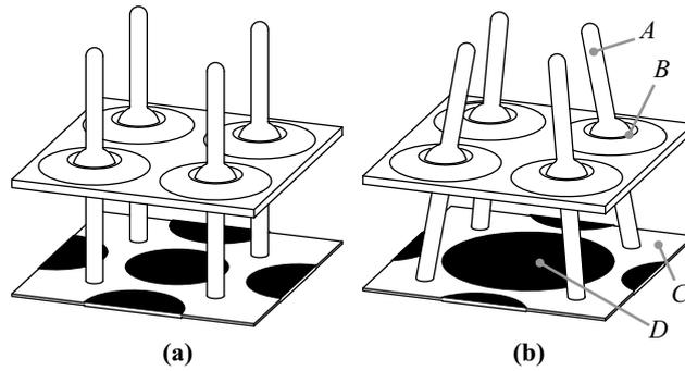
**Figure 3.** Our proposed mechanism for laterotactile stimulation. Rigid pins (*A*) are attached to a surface with compliant spherical joints (*B*). A DEA membrane (*C*) is attached to the bottom of the pins, and the user’s finger rests against the top of the pins. The device at rest is shown in (a). Actuation of a DEA element, shown in black (*D*), causes it to expand in area which causes compression at the fingertip (b).
