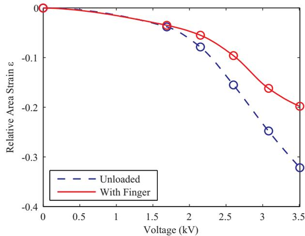
**Figure 8.** Characterisation of the relative area strain between the pins against applied voltage, in the unloaded case as well as with a finger resting on the LPD. Data points are shown as circles, with PCHIP interpolation between the data points.
