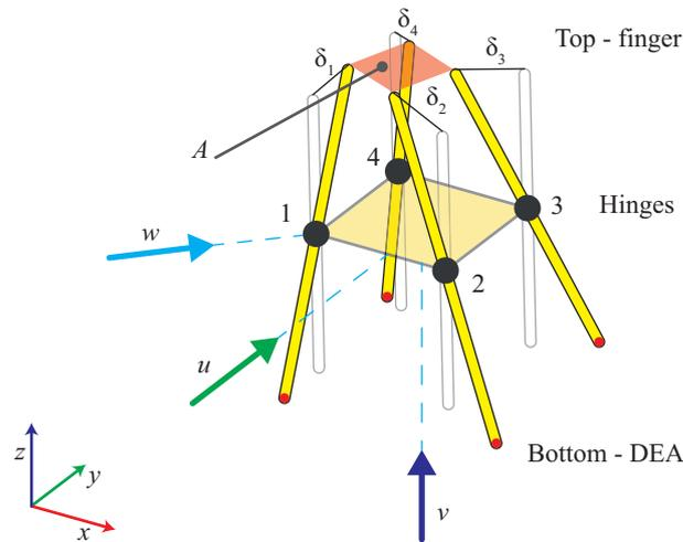
**Figure 5.** Schematic diagram of LPD mechanism, with pins numbered 1–4 and directions  $u$  (side view),  $v$  (bottom view) and  $w$  (corner view). The displacement of each pin  $i$  has been labelled  $\delta_i$ . Also labelled is  $A$ , the area enclosed by the tops of the pins.
