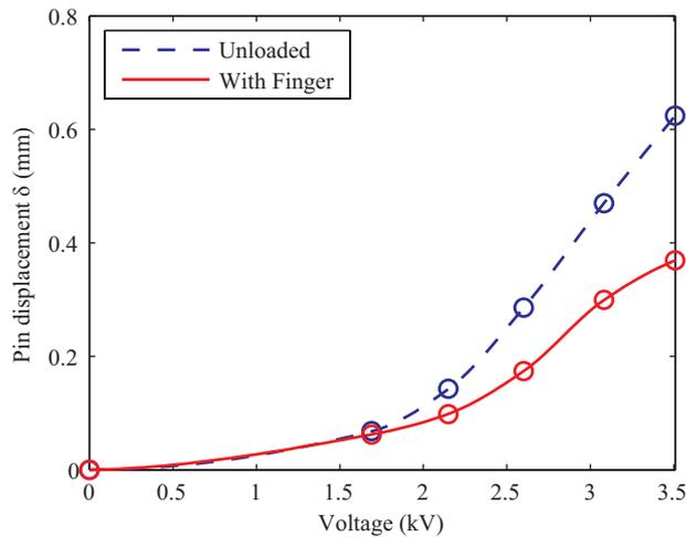
**Figure 9.** Mean displacement of the top of each pin,  $\delta$ , computed from the area enclosed by the pins in order to eliminate noise.
