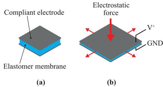
**Figure 2.** Operating principle of a Dielectric Elastomer Actuator (DEA). The DEA rest state is shown in (a). When a voltage is applied across an elastomer membrane, the electrostatic force squeezes the membrane and causes it to expand in area (b).
