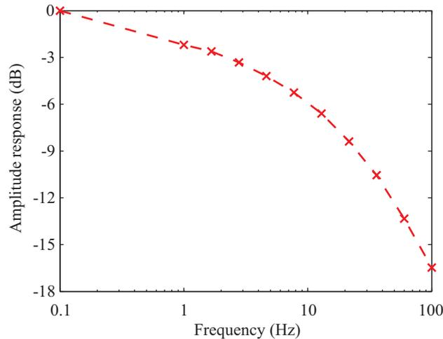
**Figure 7.** Bandwidth of LPD, with data points shown as crosses. We have taken 0 dB to be the response at 0.1 Hz.
