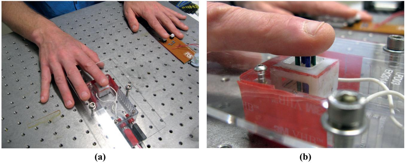
**Figure 11.** The experimental setup for the psychophysical trials. Subjects were asked to place their preferred index finger on the device but were free to press hard/lightly and have the hand open/closed to create a more realistic scenario. (a): Overview. (b): close-up view of LPD.
